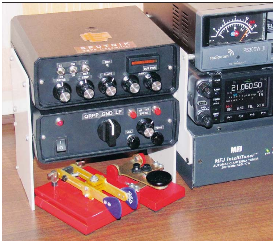
QRPP TX Sputnik 2013 with power supply, antenna switch QRPP/LP, keyer, paddle DPX-08 and key RM-Mini below, see page 16
