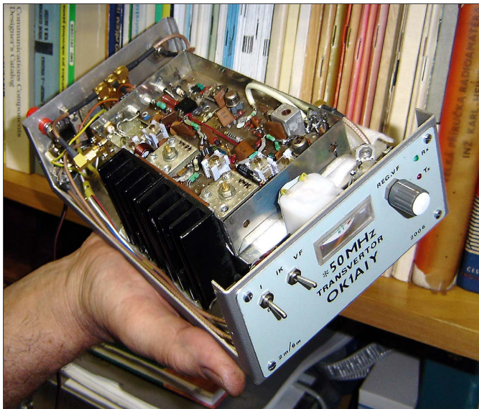
Transvertor 144/50 MHz zhotovil Pavel, OK1AIY 144/50 MHz transvertor, made by Pavel, OK1AIY
